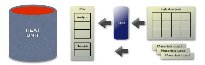
By using the software mixing tool, the operator selects the Heating Units whose analyses, together with those of the materials he wants to add, determine the expected analysis which, in real time, is compared to the material and slag specifications of the Order in process.
