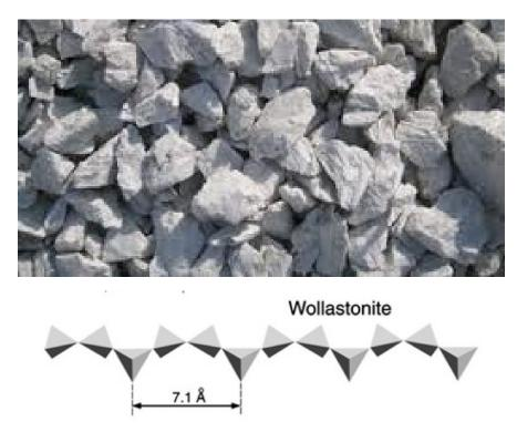
In our experiments, we employed Wollastonite in grains which, combined to lime, allowed the melting point of the slag to decrease preserving the silicon and shifting the balance of the reaction in favour of non-oxidation of chromium. (See reaction below)
